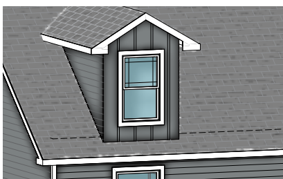
6'-0" SINGLE WINDOW CAPE COD DORMER 7/12 (non operable) or 9/12 (operable) roof only
